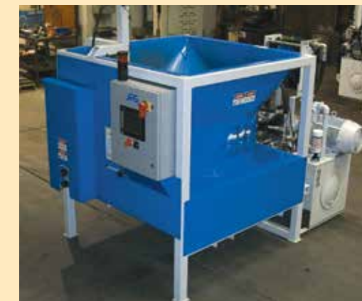
A sturdy frame of heavy-wall structural tubing protects the hopper from damage when loading. Shown with optional touch screen panel.
